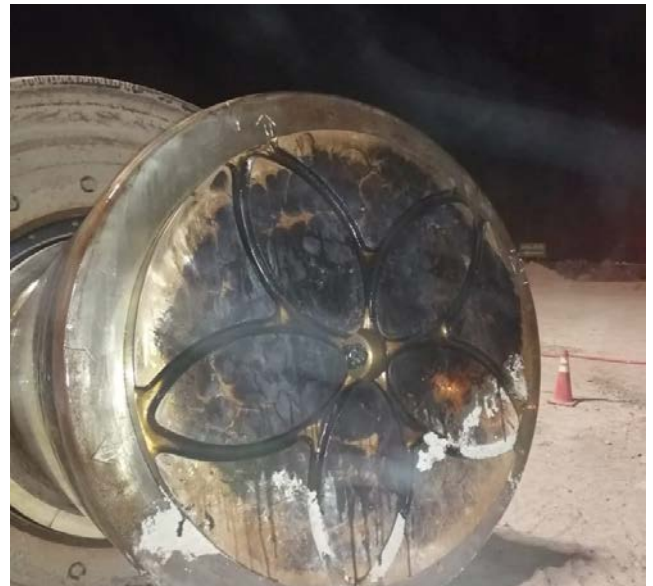
Figure 5. Scorched oil-races on base plate bearing of the mantle shaft.
